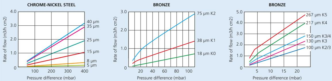
DURCHSTRÖMBARKEIT / FLOW-THROUGH / ÉCOULEMENT (V IN M<sup>3</sup>/S)
